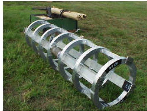
Fig. 11. Sketch and 'as-built' prototype assembly for velocity and pressure measurements on board a US Navy submarine: (a) prototype sketch; (b) 'as-built' prototype.
